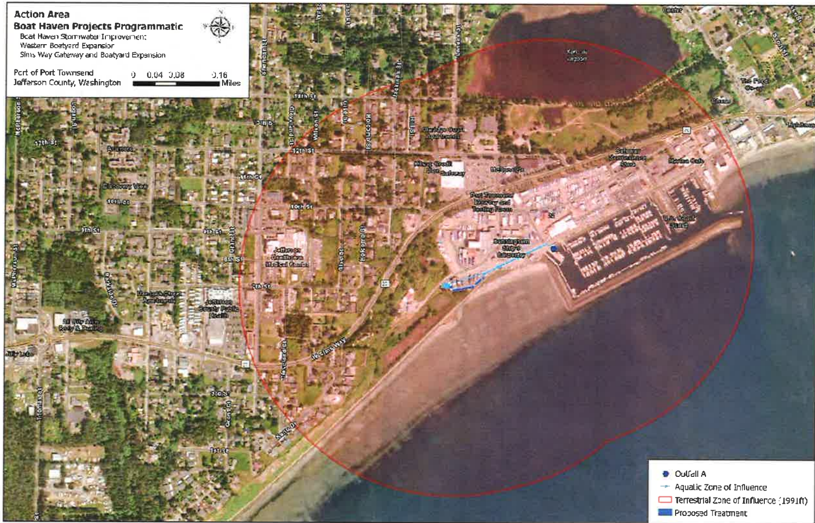
Figure 3. Action Area. The terrestrial zone of influence is defined by the extent of elevated airborne noise (1,991 feet) and the aquatic zone of influence is defined by the extent of stormwater effects.
